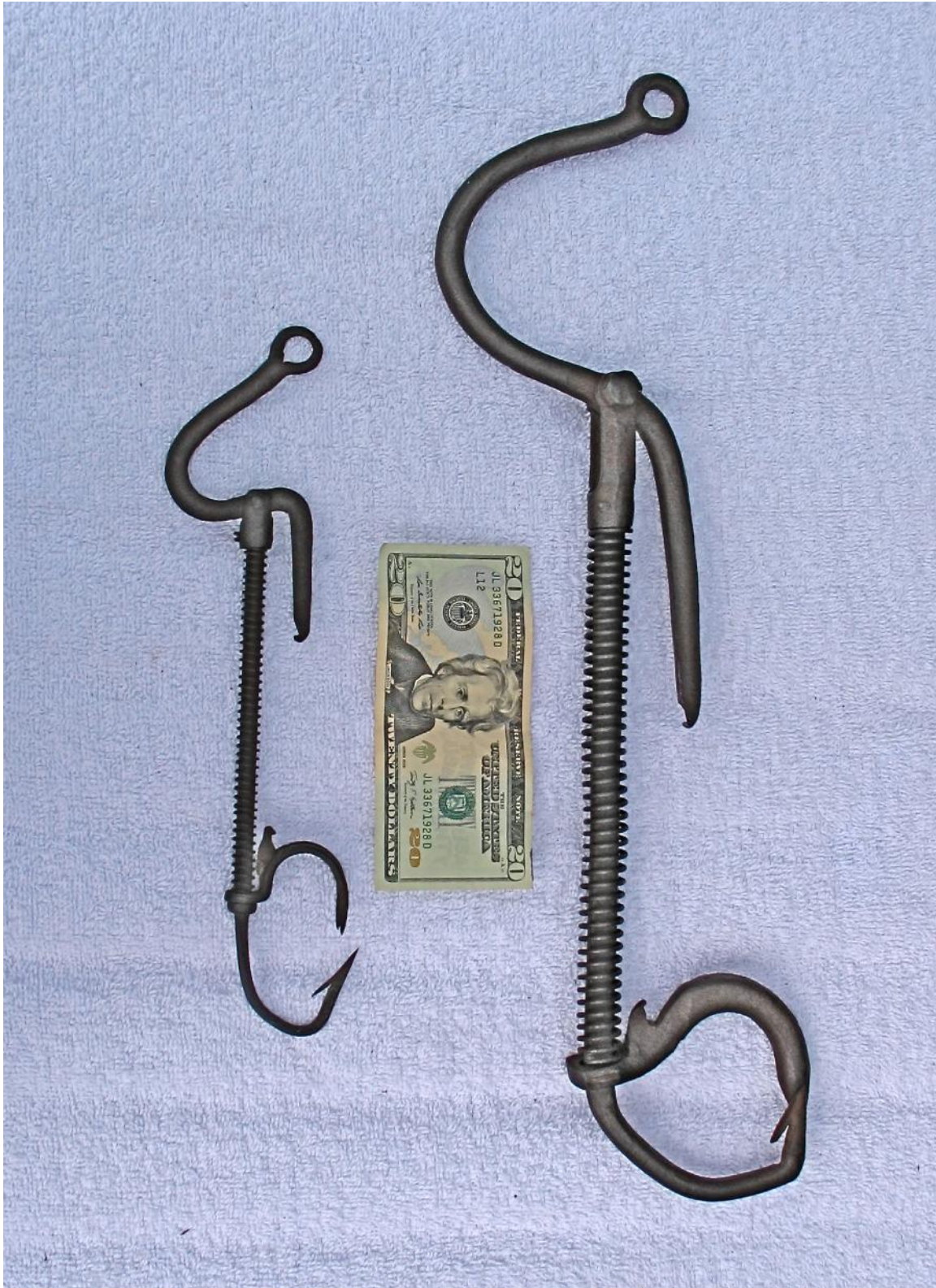
Figure 6. Von Glover Ferguson's Automatic Fishhook and his Alligator Trap shown side-by-side in a pendant orientation in the sprung position for comparison to each other.
