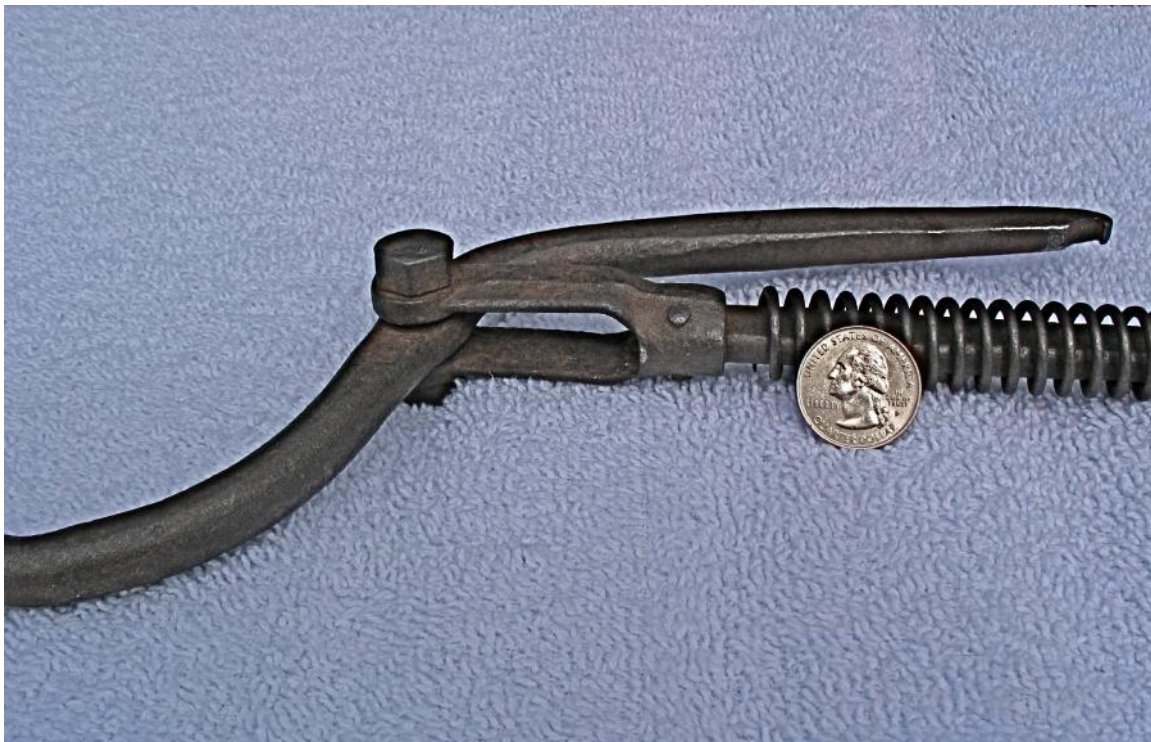
Figure 7. Close-up of the cast steel ..."bifurcated cap upon which is pivotally secured the trigger member", (the fulcrum), portion of the Alligator Trap.
